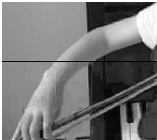
Figure 7.20 Distortion introduced by H.264 encoding (lower half)
