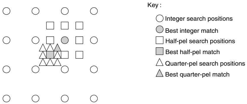
Figure 3.18 Integer, half-pixel and quarter-pixel motion estimation
